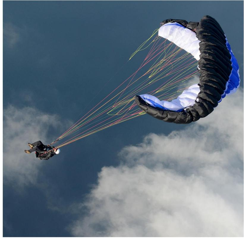
AU FUR ET MESURE QUE LA VOILE SE MET EN MARCHÉ ARRIÈRE, LES BOUTS D'AILES TRAHISSENT LE NOUVEAU SENS DU VENT RELATIF... IL VIENT DE DOS...
