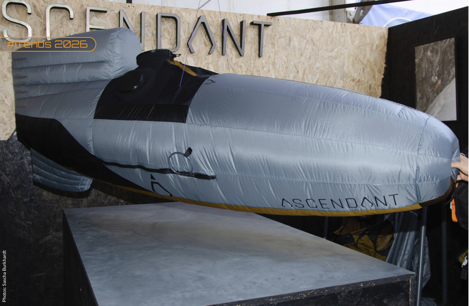
The new Calixe from Ascendant, a derivative of the Zian ST, in a public version, possibly as first pod harness. Two reserve parachutes, shorter fairing, less risk of losing visibility during a stall.
