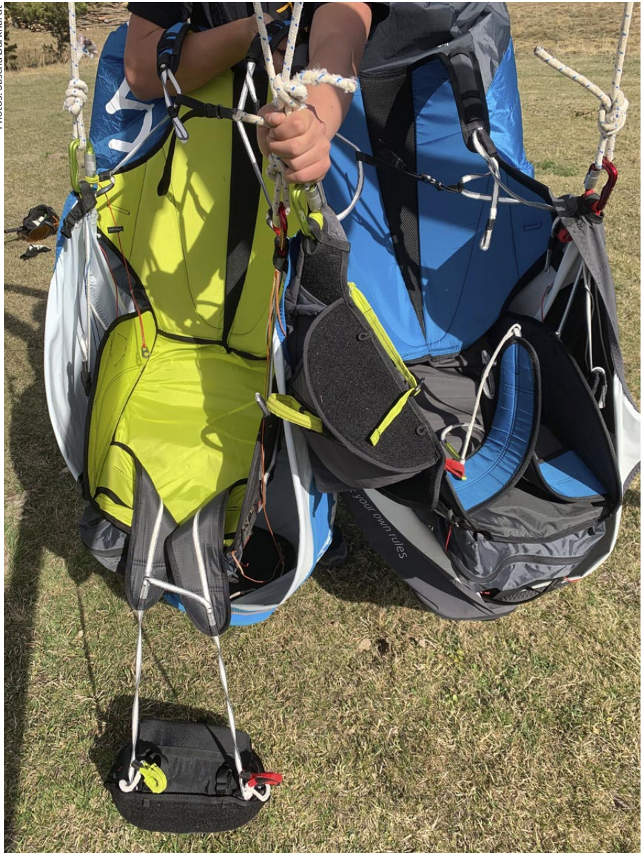
Much more practical and faster, the fastening system on the Grasshopper (on the left), vs that on the Sock (on the right), which was particularly tedious on the specimen we tested, where the buckles seemed too small.
