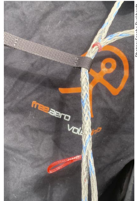
The shoulder straps are adjusted by easy to manipulate splices.
