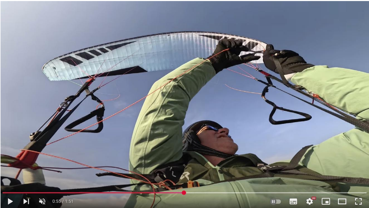
Developer Michael Nesler demonstrates that the first "A-lines" can even be cut in flight. However, these maneuver lines are considered by other manufacturers as a way to bypass EN B certification guidelines. The A-risers (labeled 3 on the left) are only used as assistance for inflation and for Big Ears. The supposed B-risers (labeled 4 on the left) are actually the "real" A-risers and extend almost to the leading edge.
